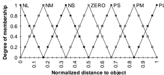
Figure 4. FNN2 - 7 fuzzy sets per input and 65 hidden layer nodes.
