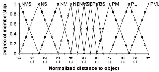
Figure 7. FNN5 - 11 fuzzy sets per input and 85 hidden layer nodes.
