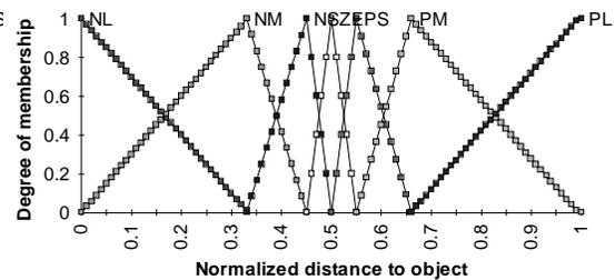
Figure 5. FNN3 - 7 fuzzy sets per input and 65 hidden layer nodes.
