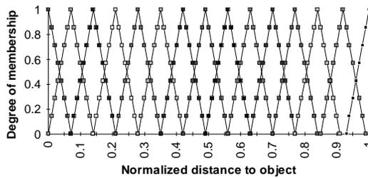
Figure 8. FNN6 - 15 fuzzy sets per input and 100 hidden layer nodes.
