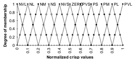
Figure 6. FNN4 - 11 fuzzy sets per input and 85 hidden layer nodes.
